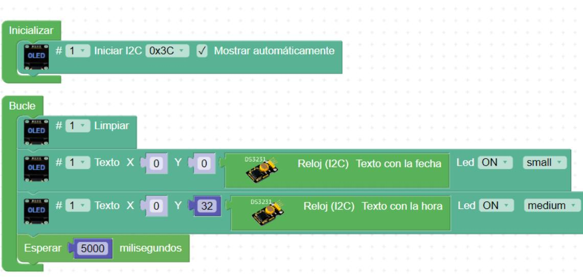
The Scratch code for displaying the RTC date and time on an OLED screen is as follows:
